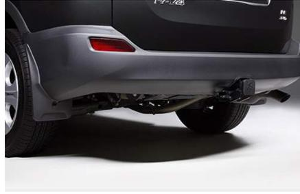
**Towing Hitch (2" Receiver), Ball Platform & Wire Harness**
