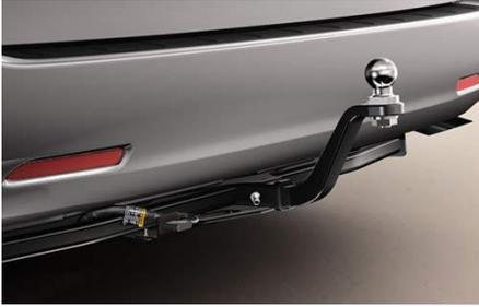
**Towing Hitch, Ball Platform & Wire Harness**
